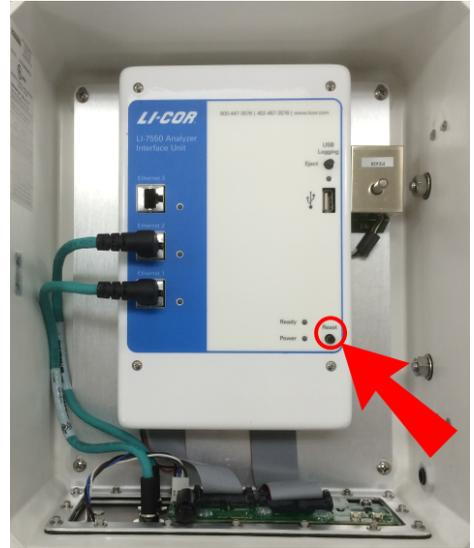
Figure 6-1. Reset button in the LI-7550.
