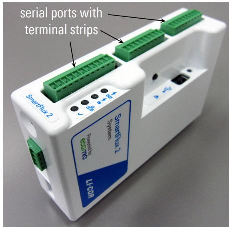
The SmartFlux 2 System comes standard with your analyzer and works with the LI-7550 Analyzer Interface Unit. It mounts inside a Biomet Enclosure, Systems Enclosure, or another suitable enclosure. This digital system includes a computer running EddyPro<sup>®</sup> software for on-site, real-time flux processing in an eddy covariance system.
