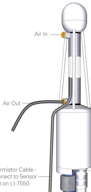
*Figure 4-1. Flow calibration gas into the calibration fitting. Attach a 15 cm (6 in.) piece of tubing to the outlet to prevent diffusion of ambient air into the calibration fitting.*
