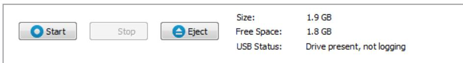
Click **Start** to begin logging data. Data logging will begin automatically when a suitable USB drive is inserted into the LI-7550 USB port and any time the instrument restarts. Press **Stop** to quit logging, and **Eject** to unmount the USB drive. Always eject the USB drive properly before removing it. After pressing the **Eject** button, the LED inside the LI-7550 will turn off when it is safe to remove the drive.
